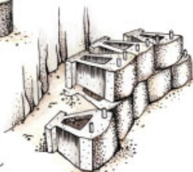
BACKFILL AS YOU GO
