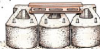
LEVELING FIRST COURSE
